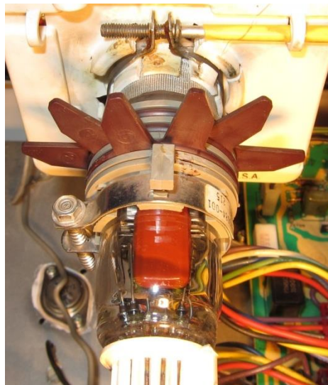
Zero-position for the CCA on a RCA 19VLUP22 CRT
