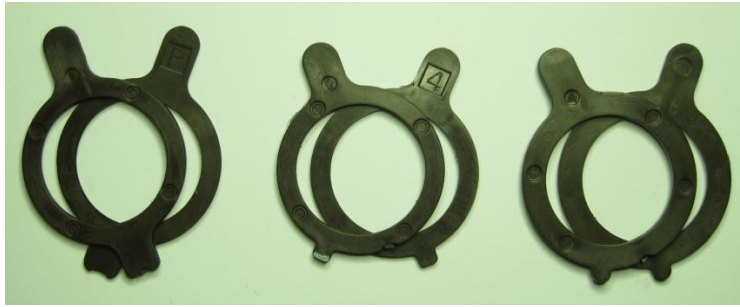
Three pair of magnetic rings (from left 2-pole, 4-pole and 6-pole)
